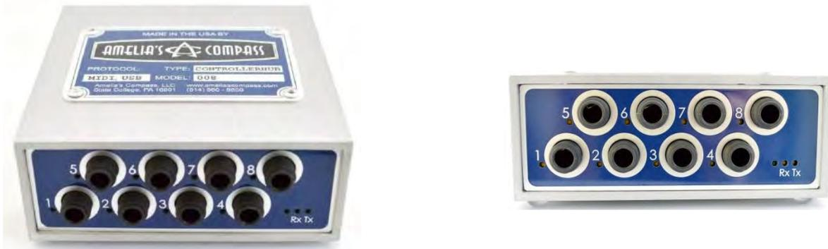
Each of these jacks enables the connection of either a variable footpedal (such as an expression pedal or some types of volume pedals) or a stomp-able footswitch (such as an on/off pushbutton, or a keyboard sustain pedal). It was a bit of an engineering challenge to allow the inputs to switch-hit between pedals and buttons, but it makes things so much easier.
