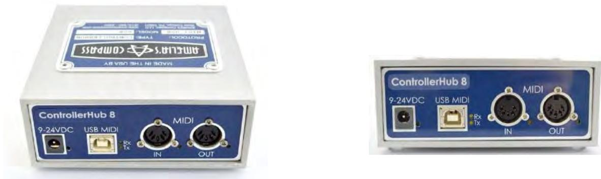
This is how you connect to the rest of your system using either USB or MIDI, whichever you're set up for. You can even use both at the same time, and this opens up some interesting possibilities which we'll get into later. Take a look at the **Combining Multiple ControllerHub 8 Units** section to find out more.
