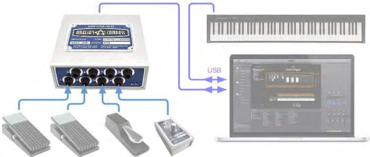
The USB keyboard and ControllerHub 8 are both connected to the laptop or tablet via USB<sup>1</sup>. The expression pedals connect to the ControllerHub 8 with 1/4" TRS cables and the buttons with standard 1/4" instrument cables.
