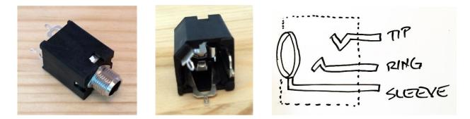
When you plug the cable connector into the panel jack, the connections are made like this:
