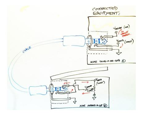
The connected equipment sends a constant, DC voltage to the pedal via the Ring connection of the TRS cable. The expression pedal returns a pedal-varied voltage via the Tip connection of the TRS. This is what the connected equipment expects, so we're in business.
