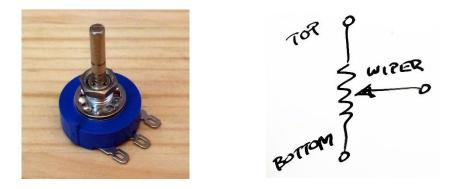
As you turn the shaft, the wiper moves up and down the length of the resistor, effectively splitting the resistor into two pieces of varying sizes, like this:
