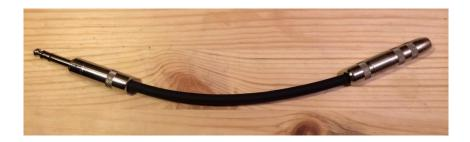
The adapter cable has 3 wires: white, black, and shield. The shield is connected to the Sleeve on both ends. But on one end the white wire is connected to the Tip, while the black wire is connected to the Tip at the other end. If the pedal has an attached cable, this adapter simply gets added to the end of it. If the pedal has a detachable cable, on the other hand, then the adapter can be attached at either end. Click here to purchase one from our website.
